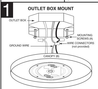
Thread 1" long mounting screws (A) into outlet box. Be sure to leave enough of the screw extended to allow the attachment of the canopy (B).
