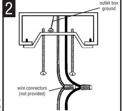
CONNECT THE WIRES. NOTE: Attach black fixture wire to black supply wire, white fixture wire to white supply wire. Do not mix them up. Use approved wire connectors (not provided).
