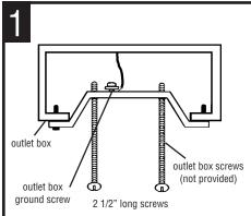
Screw green ground screw into threaded hole on cross bar between dimples. Do not tighten. Form a loop in ground wire from outlet box, place loop under head of ground screw and tighten. Insert outlet box screws (not provided) through oval slots in cross bar and attach to outlet box. Screw 2 1/2" long screws into the outer most threaded holes.
