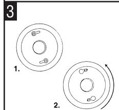
INSTALL canopy to ceiling. Push fixture wire into outlet box. Align head of mounting screws with large end of key hole slots, push canopy towards ceiling. Rotate canopy counterclockwise and tighten screws.
