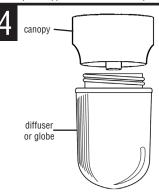
Insert light bulb into socket. Be sure to use bulb with wattage no greater than specified for this fixture. Thread diffuser into canopy. WARNING: RISK OF FIRE. MOST DWELLINGS BUILT BEFORE 1985 HAVE SUPPLY WIRE RATED 60°C. CONSULT A QUALIFIED ELECTRICIAN BEFORE INSTALLING.
