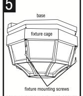
SCREW LIGHT BULB(S) INTO SOCKET. Be sure to use bulb with wattage no greater than specified for this fixture. Align holes in cage with holes in base and secure with fixture mounting screws provided.
