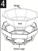
INSTALL LENSES into cage. Lower lens into fixture cage, making sure to align mounting screw holes.
