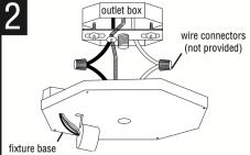
CONNECT THE WIRES. NOTE: Attach the black fixture wire to black supply wire, and the white fixture wire to white supply wire. Do not mix them up. Use wire connectors (not provided). Connect the ground wires as shown below. NEVER CONNECT GROUND WIRE TO BLACK OR WHITE POWER SUPPLY WIRES.
