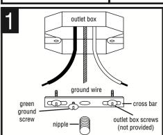
ATTACH CROSS BAR to outlet box with outlet box screws (not provided). THREAD NIPPLE into cross bar. Adjust nipple to proper height for mounting fixture.
