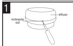
Remove the Diffuser. Insert a flat bladed screw driver into the rectangular slot and rotate the blade. The Diffuser will then pop out.
