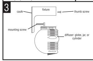
POSITION THE FIXTURE over the outlet box and secure in place with the mounting screw (provided). Screw bulb into socket. If diffuser neck is fitter type insert diffuser into fixture and tighten thumb screw into neck of globe. If diffuser neck is threaded type, screw diffuser into fixture. Thumb screw is not required. NOTE: Fixture MUST be caulked with an acrylic caulk where the base of the fixture meets the mounting surface. This provides a water tight seal when the fixture is installed.
