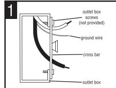
ATTACH the cross bar to the outlet box with outlet box screws (not provided).
