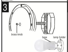
POSITION THE FIXTURE over the nipple and secure in place with brass knob. Fixture may be mounted to ceiling or wall. The photo sensor must be orientated down when the fixture is mounted to a wall. Align and insert the round ended pins on the bottom of the self ballasted lamp into the circular opening in the lamp holder key hole slots. Grasp base and rotate clockwise. Be sure to use SBCFL with wattage no greater than specified for this fixture.
