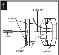
ATTACH crossbar to outlet box with outlet box screws (8-32  $\times$  1/2, 2 slotted screws NOT provided). THREAD nipple into cross bar.
