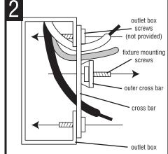
THREAD fixture mounting screws (provided) into outer cross bar. ATTACH cross bar to outlet box with outlet box screws (not provided).
