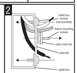
THREAD fixture mounting screws (provided) into outer cross bar. ATTACH cross bar to outlet box with outlet box screws (not provided).
