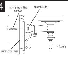
POSITION THE FIXTURE HOUSING over the fixture mounting screws and secure in place with the thumb nuts provided
