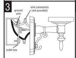
CONNECT THE WIRES. NOTE: Attach black fixture wire to black supply wire, white fixture wire to white supply wire. Do not mix them up. Use approved electrical tape or wire connectors (not provided). Connect bare fixture ground wire from outlet box. NEVER CONNECT GROUND WIRE TO BLACK OR WHITE POWER SUPPLY WIRES.
