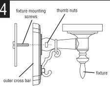
POSITION THE FIXTURE HOUSING over the fixture mounting screws and secure in place with the thumb nuts provided
