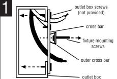
THREAD fixture mounting screws (provided) into outer cross bar. ATTACH cross bar to outlet box with outlet box screws (not provided)
