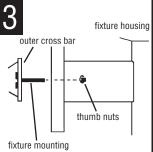
screws POSITION FIXTURE HOUSING over the fixture mounting screws and secure in place with thumb nuts provided. NOTE: Fixture must be caulked with an acrylic caulk where fixture housing meets mounting surface. This provides a water tight seal when fixture is installed.
