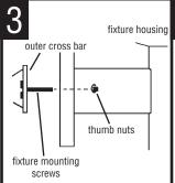
POSITION FIXTURE HOUSING over the fixture mounting screws and secure in place with thumb nuts provided. NOTE: Fixture must be caulked with an acrylic caulk where fixture housing meets mounting surface. This provides a water tight seal when fixture is installed.
