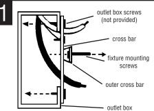
THREAD fixture mounting screws (provided) into outer cross bar. ATTACH cross bar to outlet box with outlet box screws (not provided).
