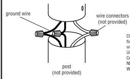
CONNECT THE WIRES. NOTE: Attach the black fixture wire to the black supply wire, the white fixture wire to the white supply wire. Do not mix them up. Use approved wire connectors (not provided). Connect bare fixture ground wire to supply ground. NEVER CONNECT GROUND WIRE TO BLACK OR WHITE POWER SUPPLY WIRES.
