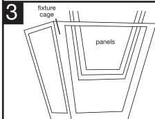
BEFORE SNAPPING HOUSING SHUT, install plastic panels, textured or beveled side out, by sliding panels down cage in slots on inside of cage. Make sure panels are all the way down into seats in cage. Some panels may fit tighter than others and a moderate amount of force may be required to install.
