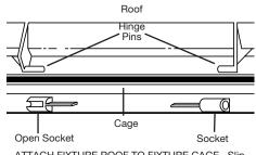
ATTACH FIXTURE ROOF TO FIXTURE CAGE. Slip one hinge pin on roof into hole in socket on cage and snap other hinge pin into open socket.
