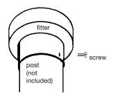
**POSITION THE FIXTURE** over post as shown. Fasten with screw at hole in post collar by drilling hole at same location through post and securing with screw (provided).
