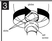
INSTALL LIGHT BULB into socket. Be sure to use bulb with wattage no greater than specified for this fixture. Attach globe to fitter by aligning dimples in fitter with slots in globe. Rotate globe clockwise. Install set screw.
