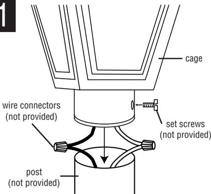
CONNECT THE WIRES. NOTE: Attach the black fixture wire to the black supply wire, the white fixture wire to the white supply wire. Do not mix them up. Use approved wire connectors (not provided).
