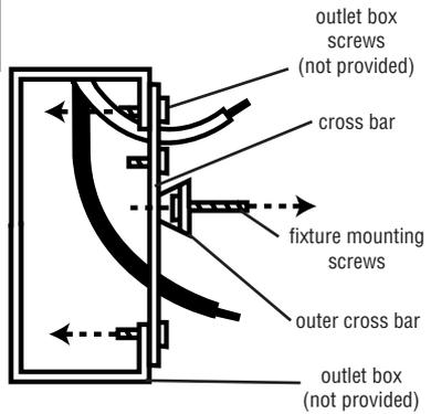
THREAD the fixture mounting screws (provided) into the outer cross bar.
