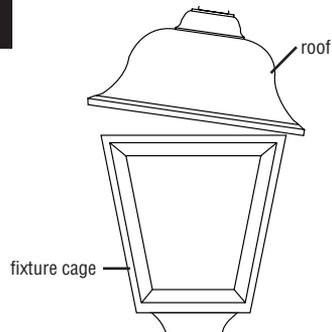
SCREW LIGHT BULB INTO SOCKET. Be sure to use bulb with wattage no greater than specified for this fixture. Lower roof and snap into place.
