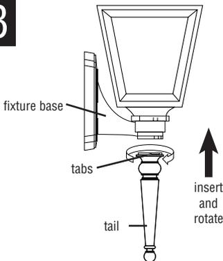
Align two tabs on tail with two notches on base. Insert tail into base and rotate tail clockwise 90 degrees.
