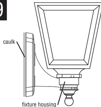
NOTE: Fixture **MUST** be caulked with an acrylic caulk where fixture housing meets mounting surface. This provides a water tight seal when fixture is installed.
