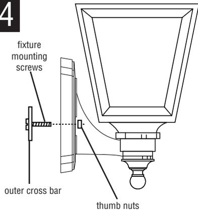
POSITION THE FIXTURE HOUSING over the fixture mounting screws and secure in place with the thumb nuts provided.
