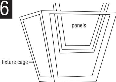
BEFORE SNAPPING HOUSING SHUT, install plastic panels, textured or beveled side out, by sliding panels down cage in slots on inside of cage. Make sure panels are all the way down into seats in cage. Some panels may fit tighter than others and a moderate amount of force may be required to install.
