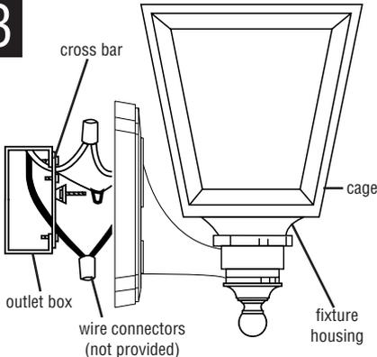
CONNECT THE WIRES. NOTE: Attach the black fixture wire to the black supply wire, the white fixture wire to the white supply wire. Do not mix them up. Use approved wire connectors (not provided).
