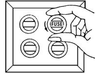
Screw-in type fuses - unscrew the fuse or fuses that control the power to the fixture or room you are working in.
