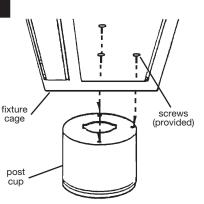
FASTEN THE CAGE to the post cup with the 3 screws provided.
