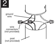
CONNECT THE WIRES. NOTE: Attach black fixture wire to black supply wire, white fixture wire to white supply wire. Do not mix them up. Use approved electrical tape or wire connectors (not provided). Connect bare fixture ground wire to ground wire from outlet box. NEVER CONNECT GROUND WIRE TO BLACK OR WHITE POWER SUPPLY WIRES.
